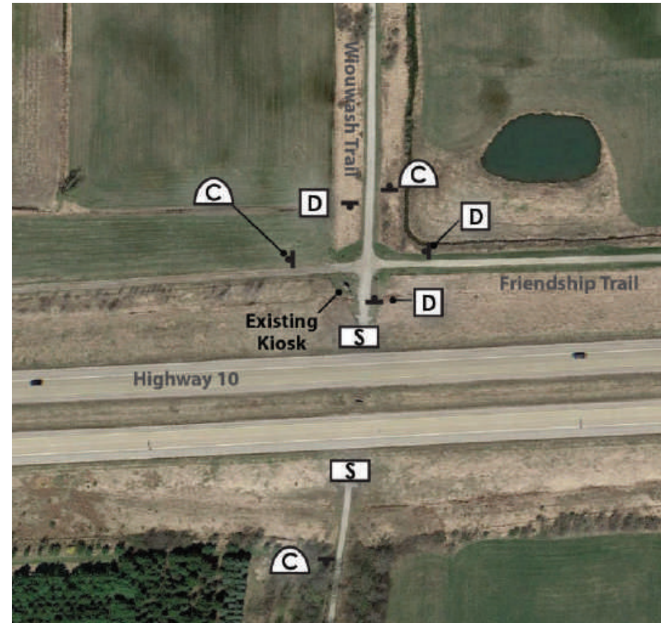
Figure 39. Decision (D), Confirmation (C), and Street name (S) sign placement at a trail underpass and trail intersection.
