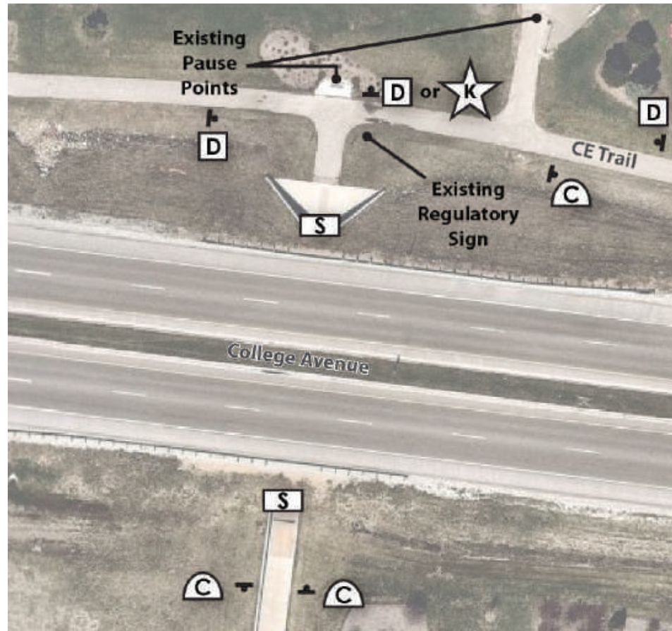
Figure 38. Decision (D), Confirmation (C), Street name (S), and Kiosk (K) sign placement at a trail underpass and destination spur.
