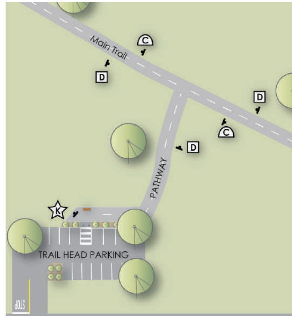
Figure 33. Typical Decision (D), Confirmation (C), Turn (T), and Kiosk (K) sign placement at trailhead spur trails.
